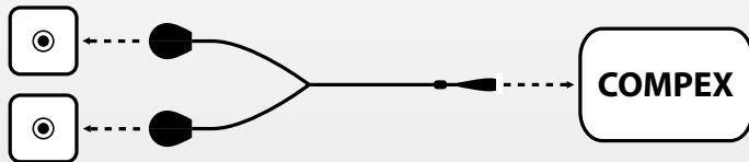
N.B. The MI-sensor cable (if available with the device) can be connected to any socket on the stimulator.
